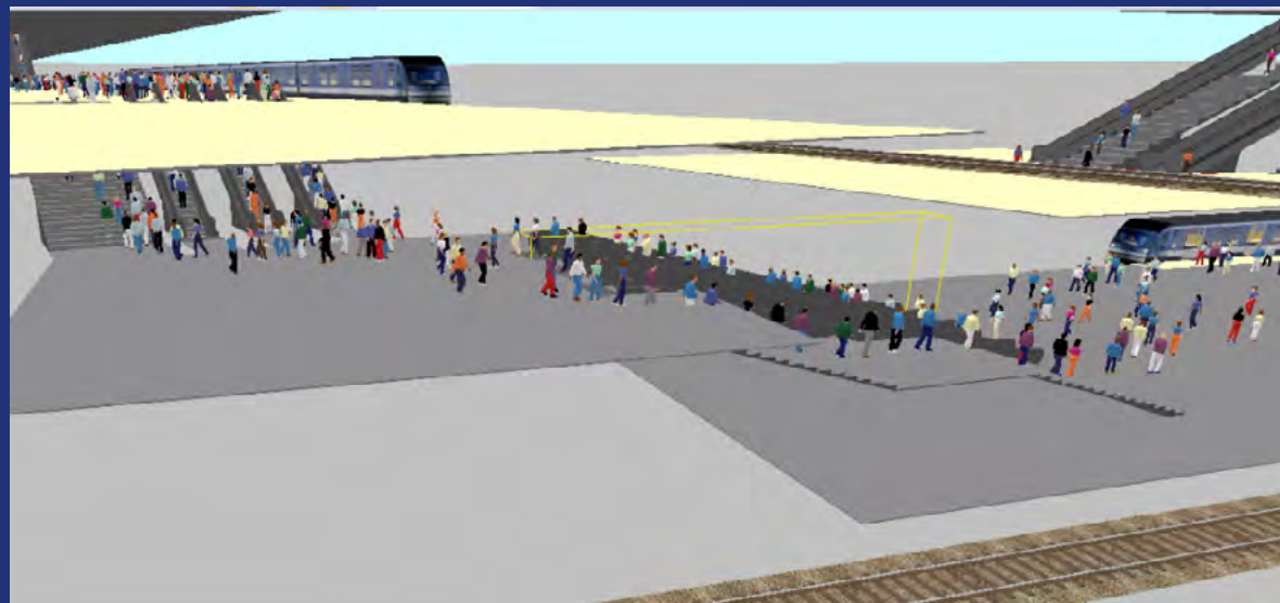
The shortest path between both platforms: in these cases, the passengers on relevant routes could be instructed to use the wagons at the edges of the trains in order to shorten their walk.
